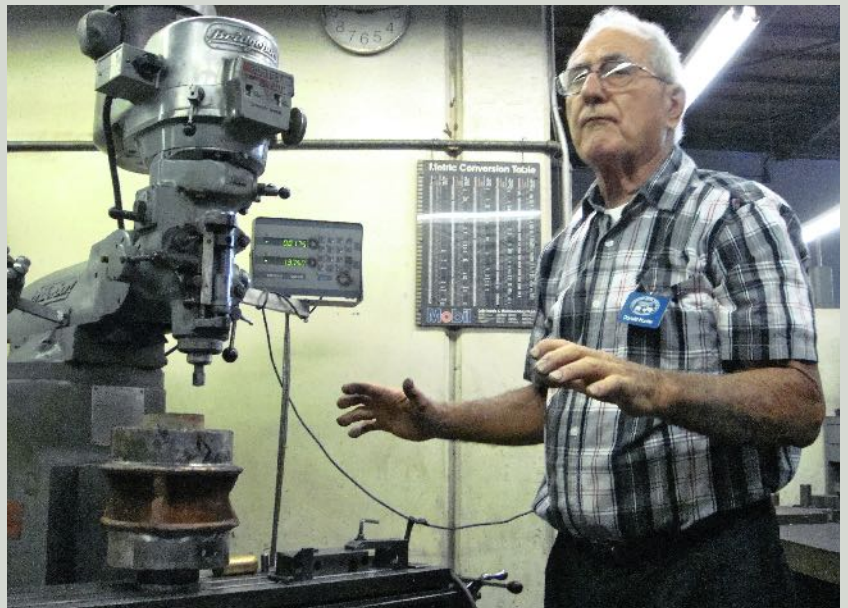
Don demonstrates a technique for machining large track rollers
