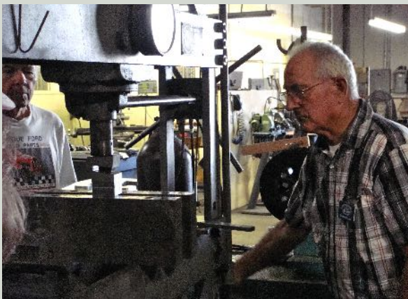
Straightening in a press requires proper back-up
