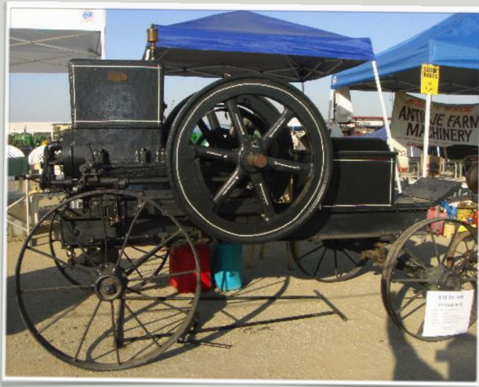
Eight horsepower Domestic engine, built in Shippensburg, Pennsylvania. This engine was shown by Mike and Gloria Jones. Domestic engines are unique in that the exhaust valve and ignitor are operated off of a sideshaft.
