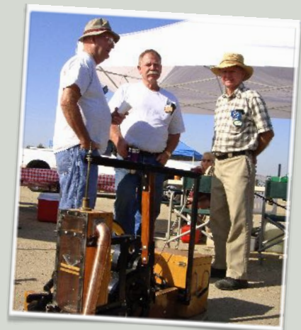
Larry Evans, Mike Jones and Ken Evans debating the subtle characteristics of Ken's eight-cycle Aermotor. The engine can only fire once every 1440 degrees of crankshaft rotation.
