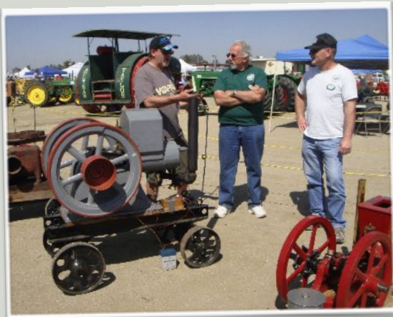
Craig Mathews explains his St. Mary's engine. This engine's exhaust valve operates off the pressure in the cylinder after the engine fires. Yes, it's very strange.
