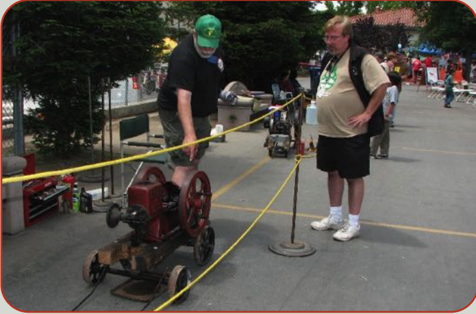
Joe Siddons explaining the operation of a hit and miss engine
