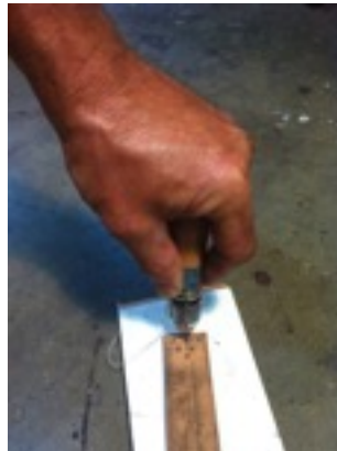
Use an awl to poke holes in the leather.
