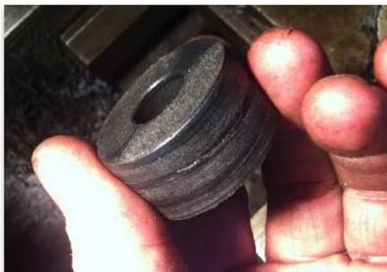
The chunk of ABS was machined into a "gear blank" with the correct inside and outside diameters, copied from the original gear.
