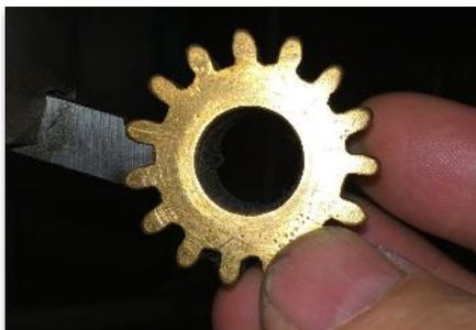
Holding the plastic "gear blank" on the milling machine was done with an indexing head. An arbor was made to fit the inside diameter of the gear blank, with a screw on the end that would hold the blank securely. The indexing head would allow the
