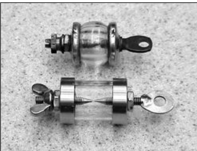
At the top is an original Meissner intensifier. At the bottom is a modern copy using an oiler sight glass.
